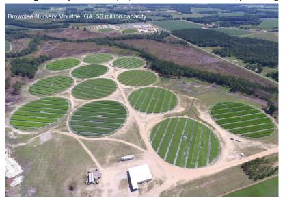
a 204' arm, which would irrigate 3 acres (see photo). Instead of reworking the old beds, grow seedlings on metal benches. Conifer seedlings can be grown at higher density in containers (40 to 70/ft<sup>2</sup>)—a second advantage over bareroot bed density. Twenty-five pivots installed on 100 acres could produce about 100 million seedlings.
